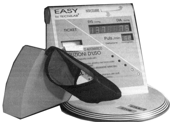
SLIKA 1: FOTOGRAFIJA ELEKTRONIČKOG TLAKOMJERA ZA KRVNI TLAK TIPO EASY
